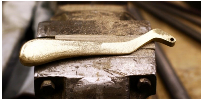
Figure 9 Filing and refining final tool
